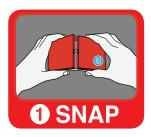
Hold the CellAED<sup>®</sup> TRAINER in both hands with the label 'Reusable Liner - Do Not Discard' facing downwards (toward the "patient's" chest). Press down and inwards to SNAP the trainer in half. The CellAED<sup>®</sup> device liner is labelled 'This Side Face Down'.
